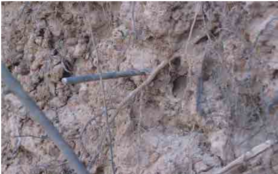
Fig. 2: Erosion Pin at the bank of the Birim River at Akim Oda (Photo by John Kusimi)
